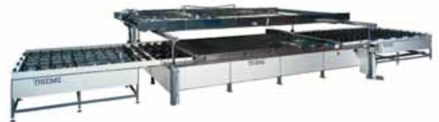
Pic.5: Printhead in screen cleaning position, moved 1200 mm towards the rear
